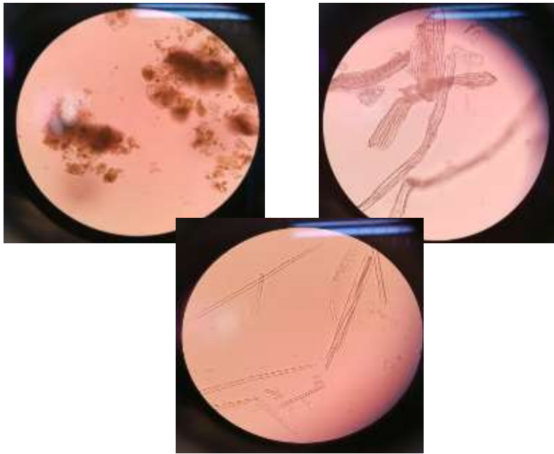
Figure 3: Images which observed under light emission microscope with x100 magnification for: (a) raw materials in powder form; (b) samples after chemical treatment and (c) samples after bleaching.
